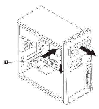
Figure 24. Removing the optical drive
